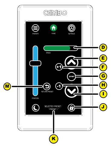
Back at the control panel note the pre-set selection indicator [K] now shows the selected pre-set and the return to pre-set button [M]. You are now able to fine tune the camera position using controls [E] to [I]. Set the desired working speed by sliding [D] left for slower or right for faster. Press +1 or -1 to make the minimal adjustment of one unit. Jump back to the pre-set position by pressing return [M].
