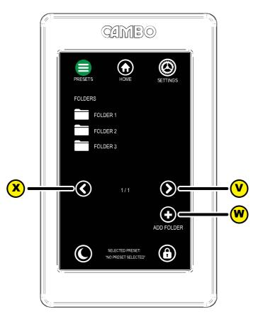
To create a new pre-set you need to select a folder from the pre-set menu. Either select an existing folder or create a new folder. navigate through the folder pages by using the arrows [V] and [X].
