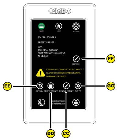
Press return [EE] to return to the pre-set list. Or press Go To [GG] to select this pre-set. If you press go to [EE] you will automatically jump back to the control panel, the cross-arm will move to the height saved by the pre-set. Press Go to [GG]
