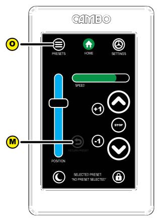
After finishing the automatic calibration the control panel opens. The RPS-system is ready for use. Notice the return to pre-set button [M] is greyed out by default. This is because there is no pre-set height selected. To select a pre-set or create a new presets based on the current cross-arm height, press the pre-set menu button [O].
